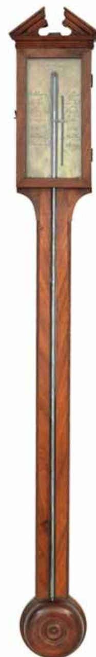
471 A GEORGE III MAHOGANY STICK BAROMETER The dial engraved 'Robb Montrose' The brass dial with visible tube and adjustable vernier, the feather banded body above a circular cistern, 14cm wide, 6cm deep, 98cm high, (5 1/2 in wide, 2in deep, 38 1/2in high) £300 - 400 €330 - 440
